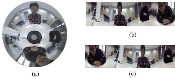
Fig. 1. A donut-type image (a) captured by ODC and two un-warped images (b) and (c) from image (a) with different baselines
