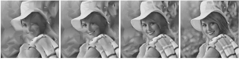
Fig. 7. Example of level-of-detail control on the “Elaine” image. Beginning from left to right, \delta_{w1} is set to 80, 60, 40, and 20, respectively.
