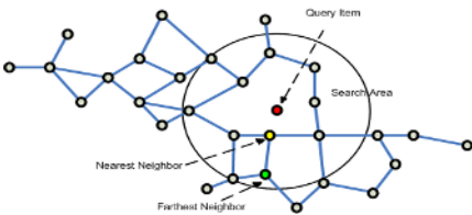
Fig. 2. Illustration of the first step of the local updating method(Retrieving of the search Area)
