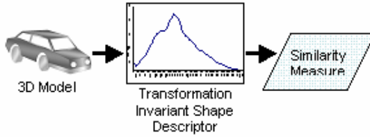
Fig. 2. Extracting a rotation, scale and translation invariant shape descriptor from a 3D model
